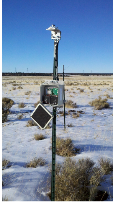
Figure 3.2: Each irradiance sensor used in the study was mounted on a fence post and connected to a datalogger box, which was powered by a small PV panel.
